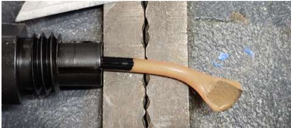
Figure 1. Thermotube Adapter Assembly in Position for Trimming
