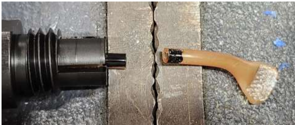
Figure 2. Example of Properly Trimmed Thermotube Output End
